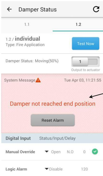
One of the possible errors, when the damper has failed to move from the position „Close“ to the position „Open“ in time
