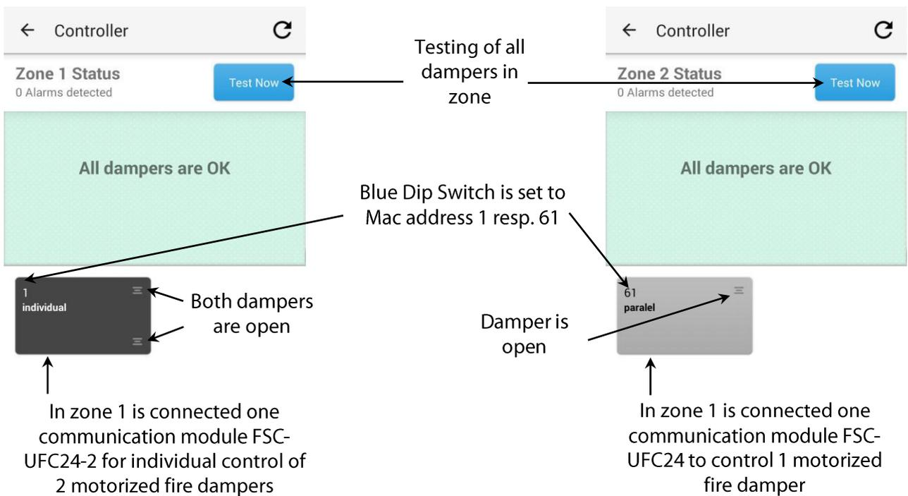
Individual control of 2 dampers on address 1 will be automatically divided into addresses 1.1 a 1.2
