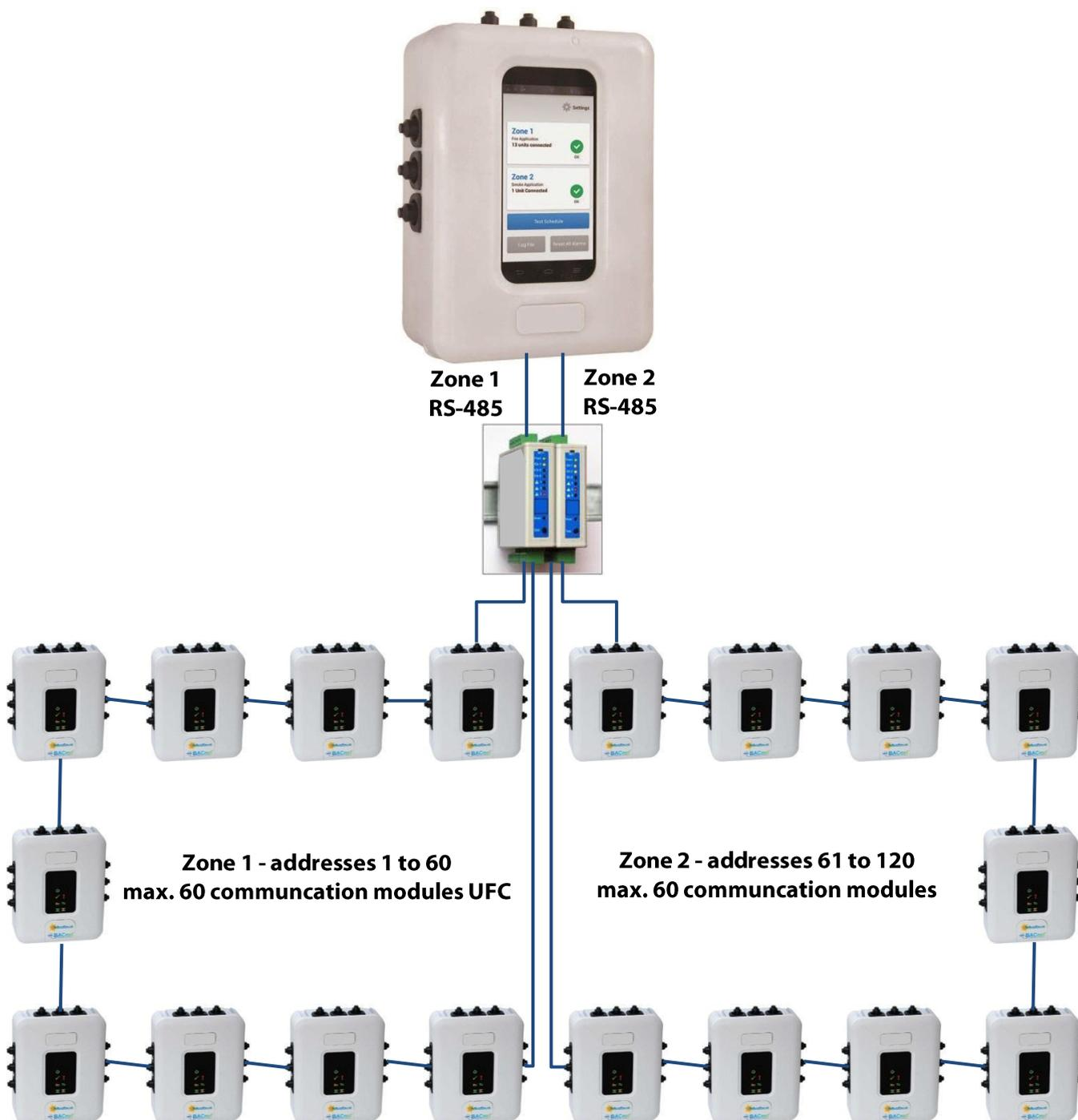
One FSC-A-RSM module is used for each zone, creating a ring topology in each zone. If communication is interrupted at any point, due to this connection we will not lose communication with the communication modules because communication can continue from the other side. When using a ring topology, it is not necessary to use the  $120\Omega$  termination, which should be switched on in the UFC communication modules when the communication module is the last one in a line.
