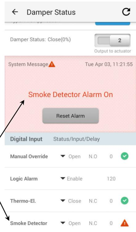
Signalization of an error, triggered by smoke detector
