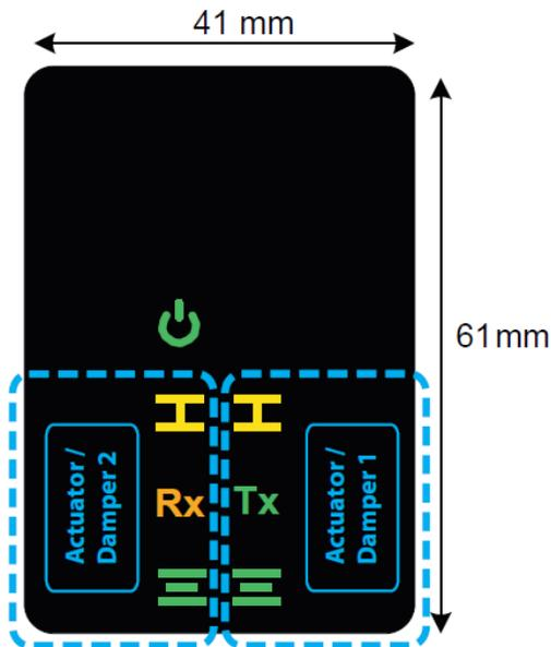
**Important:** If only one actuator is connected to the FSC-UFC24-2 the LEDs of the side where no actuator is connected indicate an alarm. A jumper has to be installed between S4 and S6 in the terminal where there is no actuator connected, to indicate an “opened” position in the LED. If the second connection is not activated via bus, there will be no alarm signal on the bus system.
