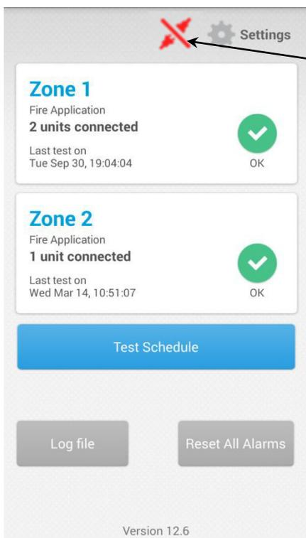
This symbol will appear when the connection between the screen and the central control module is interrupted
