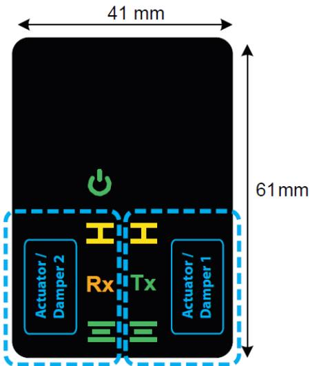
**Important:** If only one actuator is connected to the FSC-UFC230-2 the LEDs of the side where no actuator is connected indicate an alarm. A jumper has to be installed between S4 and S6 in the terminal where there is no actuator connected, to indicate an “opened” position in the LED. If the second connection is not activated via bus, there will be no alarm signal on the bus system.
