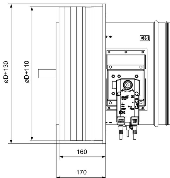
**In solid wall construction - installation frame R3, R4**
