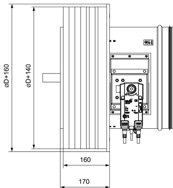
In solid wall construction - installation frame R1, R2
