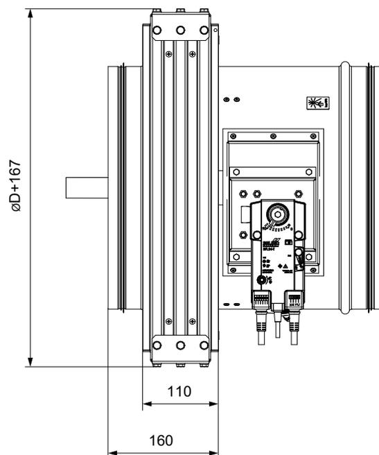
In solid wall construction - installation frame R5
