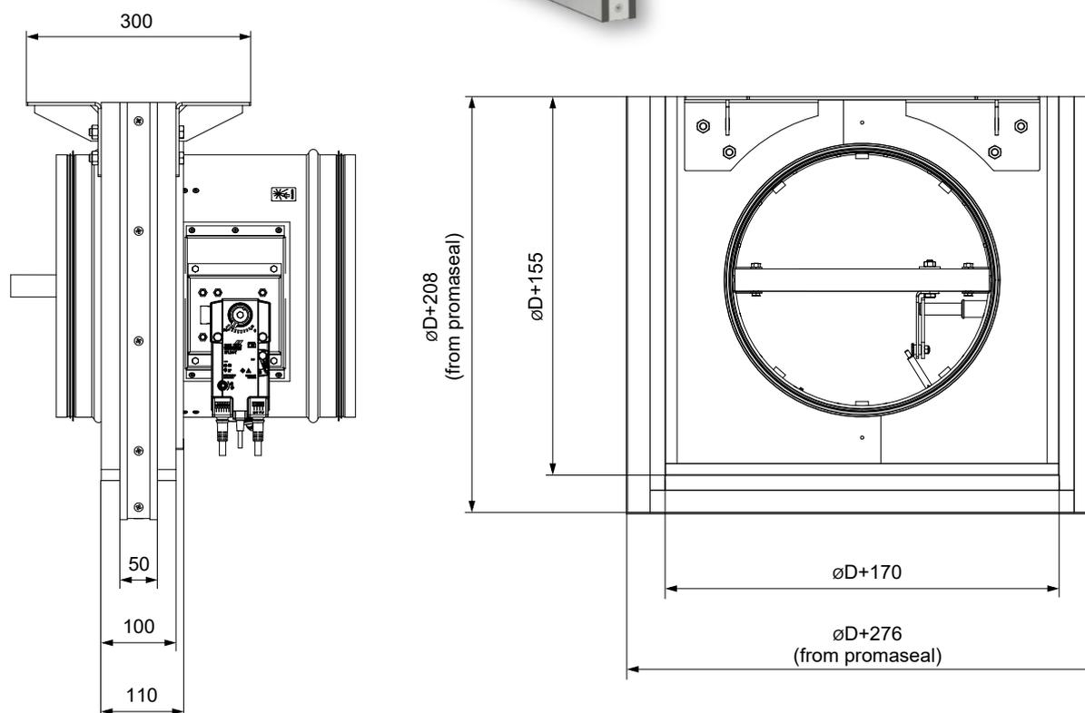
In gypsum wall construction - flexible ceiling - installation frame R7
