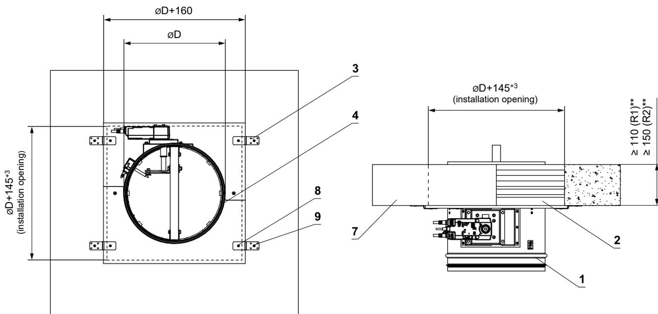
\*\* min. 110 mm - Concrete - for EI 90 S - Installation frame R1
