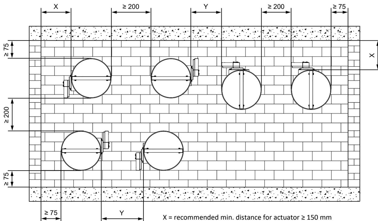
X = recommended min. distance for actuator  $\geq 150$  mm
