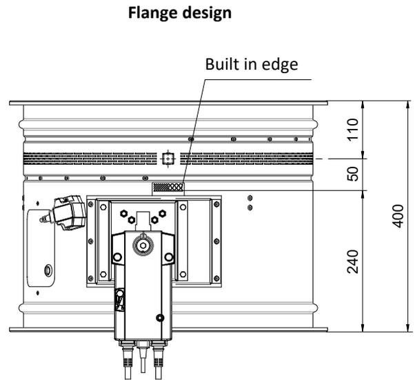
"BUILT IN EDGE label" indicates the recommended edge of installation of a fire damper in the fire separating construction (wall/ceiling). The damper must be installed so that the entire damper blade (in the closed position) is located in the fire separating construction (wall/ceiling) and at the same time the actuating mechanism and inspection openings are freely accessible.
