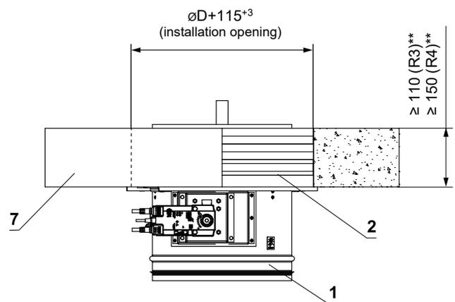
\*\* min. 110 mm - Concrete - for EI 90 S - Installation frame R3
