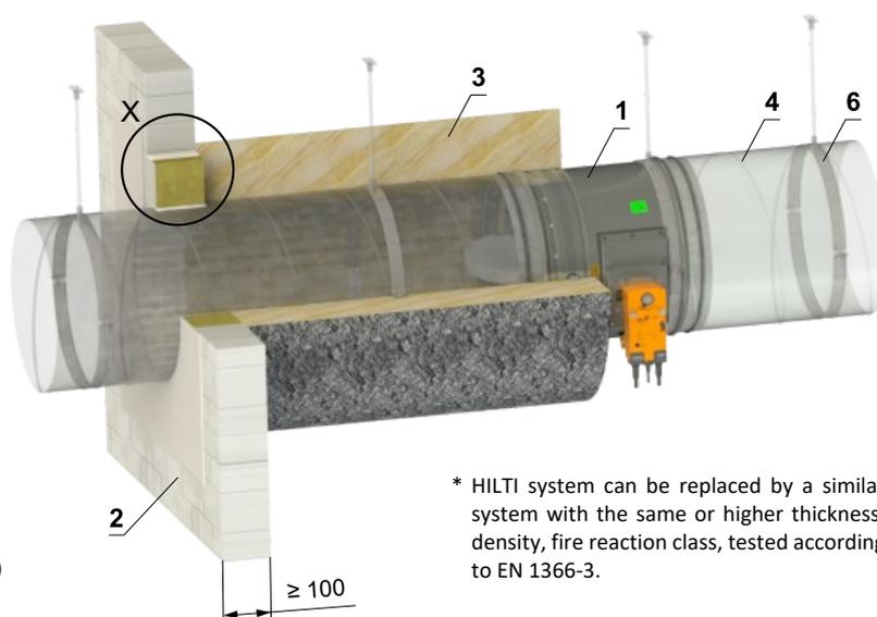
\*\* EI 60 S for DN 100 – DN 800 - thicknes 100 mm
