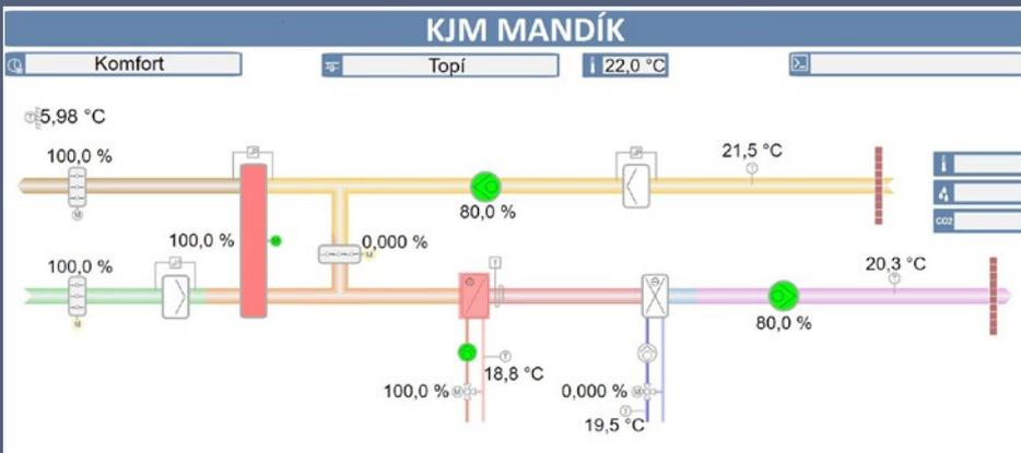
The technological diagram provides you with an overview of the status of the devices and of the internal climate, allowing you to evaluate the situation and quickly act as needed.
