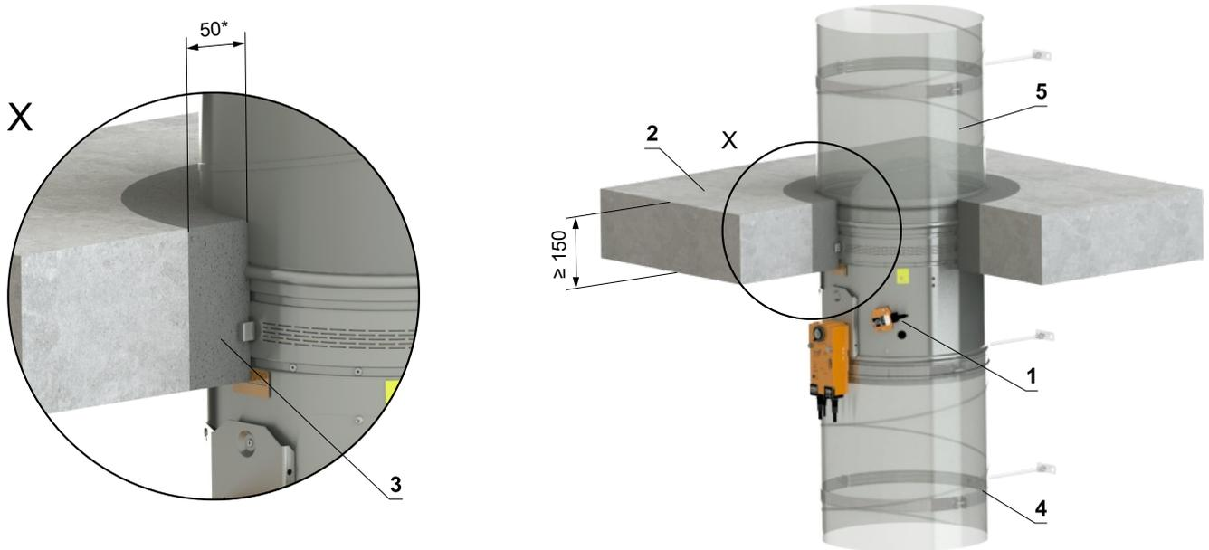
\* For fire resistance EI 45 S is approved opening between the construction and the damper in the range of 50...150 mm.
