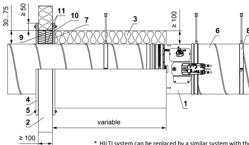
\* HILTI system can be replaced by a similar system with the same or higher thickness, density, fire reaction class, tested according to EN 1366-3.
