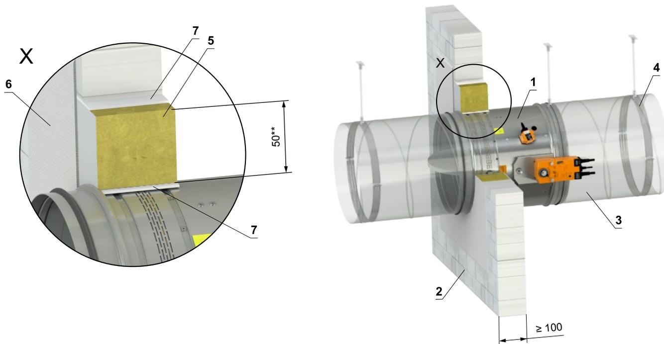
\*\* For fire resistance EI 45 S is approved opening between the construction and the damper in the range of 30...75 mm.
