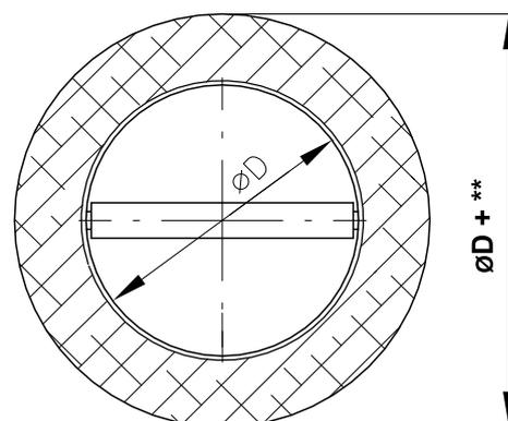
**\*\* Mortar or gypsum, damper in solid wall construction (round opening)**
