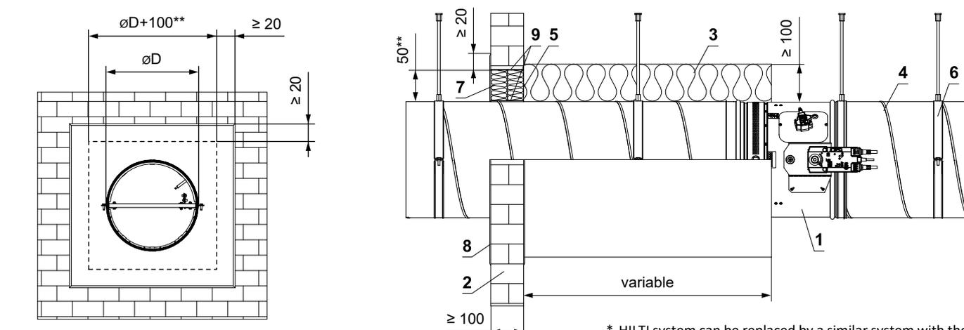
\* HILTI system can be replaced by a similar system with the same or higher thickness, density, fire reaction class, tested according to EN 1366-3.
