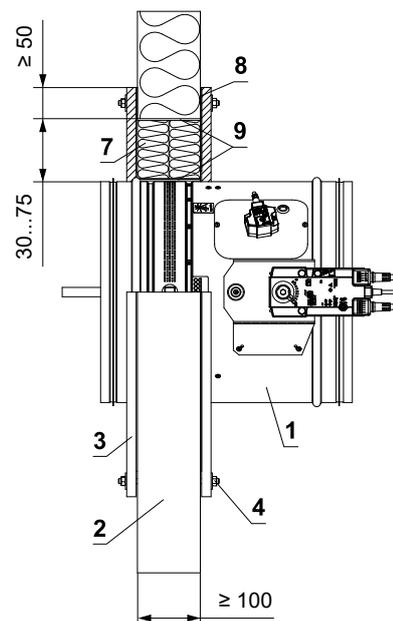
\* HILTI system can be replaced by a similar system with the same or higher thickness, density, fire reaction class, tested according to EN 1366-3.
