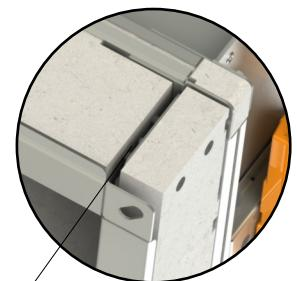
Completely fill the gaps between boards!
