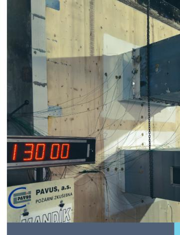
MANDÍK's FDMS and FDMB fire dampers, tested with Cross-Laminated Timber (CLT) walls and ceilings, provide top-notch fire resistance. The FDMS achieves El 60 S in 90 mm CLT walls, while the FDMB reaches EI 90 S in both 100 mm CLT walls and 140 mm CLT ceilings, making them excellent for sustainable construction.
